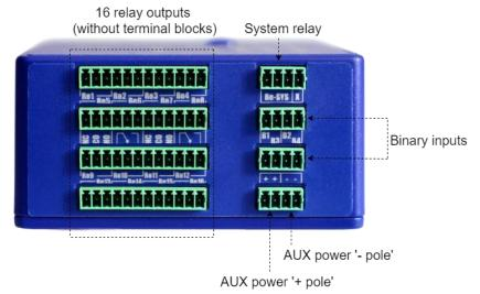
Terminal blocks are used to connect supply wire or to connect several wires together in electrical engineering. Where to connect these terminal blocks and how they look like is shown in the following picture. We connect terminal block for relay 1-4.
