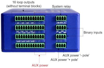
Terminal blocks are used to connect supply wire or to connect several wires together in electrical engineering. Where to connect these terminal blocks and how they look like is shown in the following picture. We connect terminal block for loop 1-4 and their powering.
