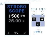
Initially the strobo uses the speed frequency (if it is known) or the last speed from memory.
