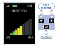
Adjust the brightness with the Arrow buttons
