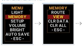
The list of saved readings appears. Every readings is described in two lines. The Point ID and value are on first line and time/date of reading on the second. Use Arrow buttons for listing.
