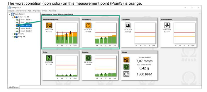
In this moment, orange color is the worst color of all measurement points on machine Motor+Fan. So, it is copied to the machine level (one level higher in the structure).
