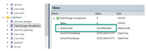
Every machine includes the same fault folders as points (see picture below). There is always shown the worst fault value on this machine (from all the measurement points on this machine).
