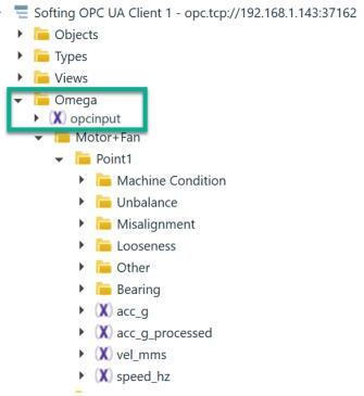
Click on '**opcinput**' in structure (directly under Omega). Double click on value 0 (green frame in the picture below – 0 is default value) and enter speed value. Press 'Enter' on the keyboard to confirm.
