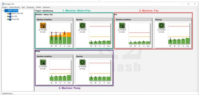
All machines (included in this project) are shown here. You can see the machine condition and the bearing condition for each machine. Let's explain how the color works for the project structure items and the icons. There is clear relation between the colors and the levels of the project structure. The worst color is copied from the 'lowest' structure parts to the 'higher'.
