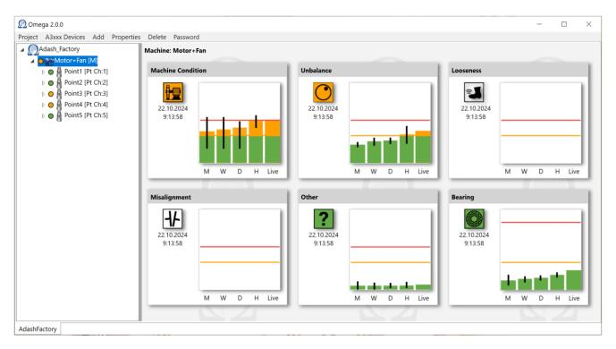
OMEGA engine itself exposes fault severity data (machine condition, unbalance, etc.) on OPC server. These values are of course displayed in Omega software.
