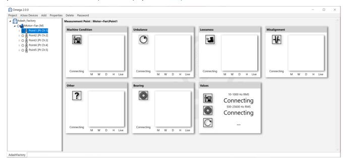
You can see that there are graphs showing information about overall machine condition, unbalance, looseness, misalignment, other and bearing values. But no bar will be shown in graphs at this moment.
