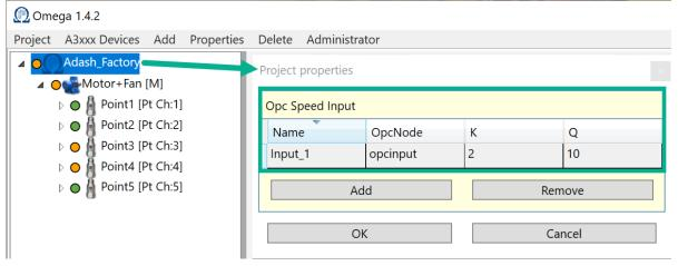
Here it is shown in OPC. Opcinput is the input value. Speed\_hz is recalculated value to Hz from the input unit.
